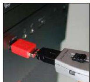
② Insert the Universal key into LINKON lock button hole. Make Universal key to (a) Pull out position and pull out the lock button
