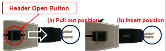
① Press "Header Open Button" all the way toward to change the key to (b) Insert position
